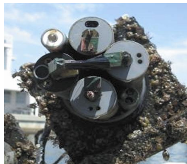
Biofouling build-up on marine data collection instruments with BioDefense 24/7™ after 150 days.
