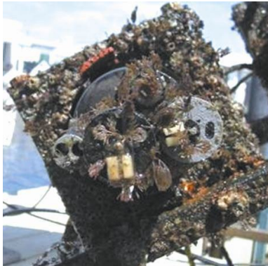
Biofouling build-up on marine data collection instruments without BioDefense 24/7™ after 30 days.
